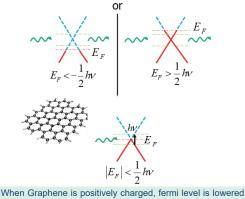
$(E_f < -h\nu/2)$ , transmission is allowed. When  $-h\nu/2 < E_f < h\nu/2$ , transmission is attenuated and the incident light can excite electron. When Graphene is negatively charged  $(E_f > h\nu/2)$ , there is no state available for the electrons to be excited to. Therefore absorption in this case is zero<sup>1</sup>.
